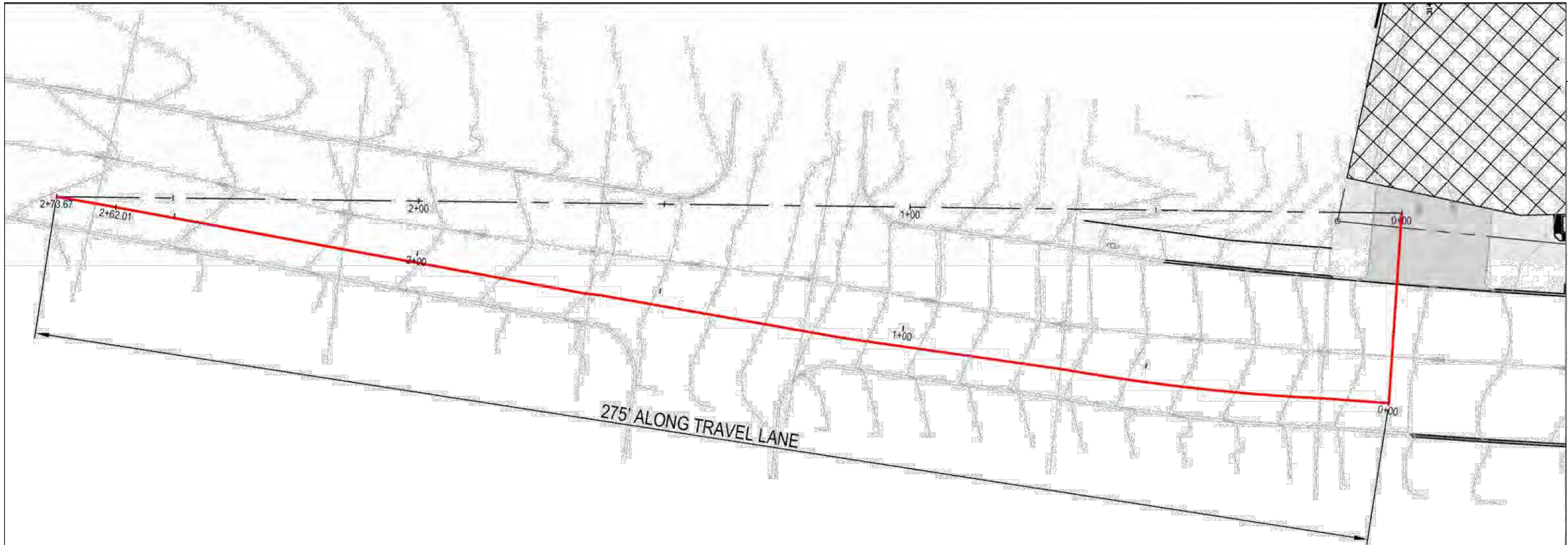
1 BEDFORD INTERSECTION SIGHT DISTANCE PLAN VIEW DATE: 4/4/2025 SCALE: 1"=20' ORIGINAL SCALE 1"=20'
