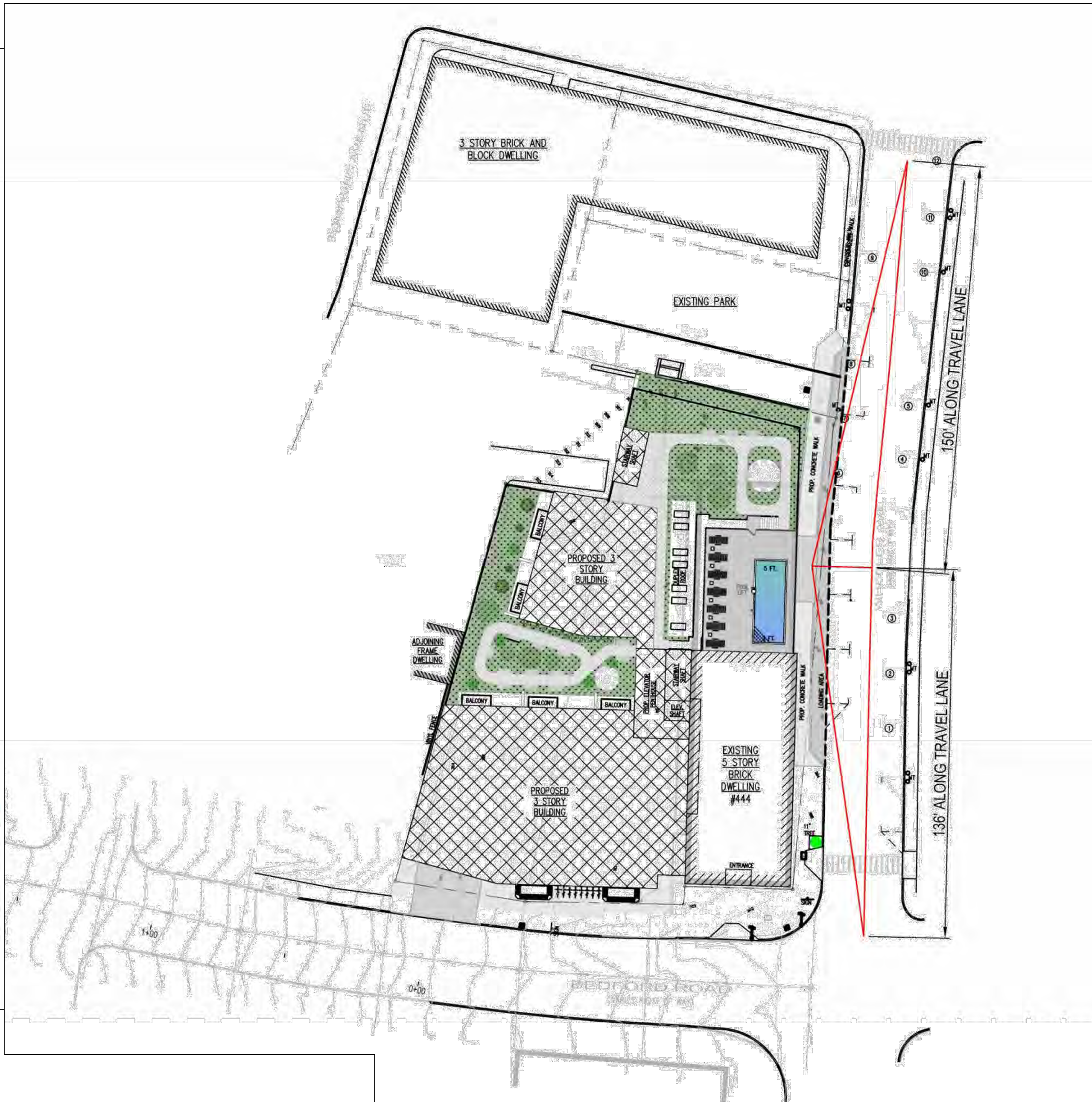
1 WHEELER AVE INTERSECTION SIGHT DISTANCE PLAN DATE: 4/4/2025 SCALE: 1"=30' ORIGINAL SCALE 1"=30'
